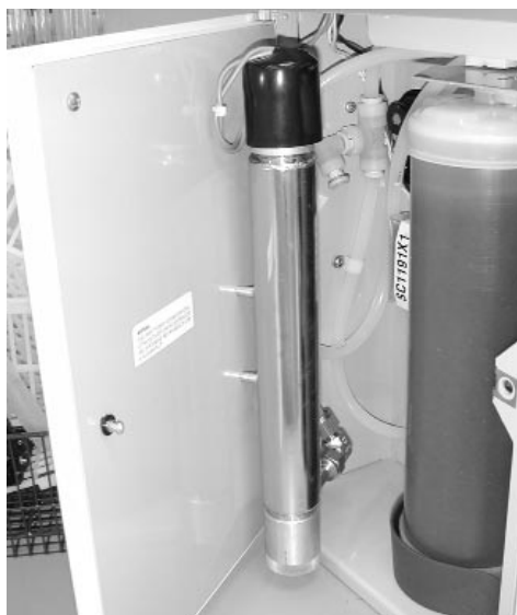
UV Lamp Installation - Left side view
